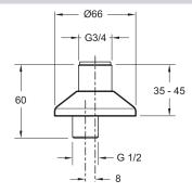
Product Specification: Pack of connectors. E75414. Collection: NO COLLECTION. WEIGHT: 0.8 kg. MATERIAL: Metal. INSTALLATION TYPE: Wall-mount.
