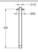
Product Specification: Arm for showerhead. E10043. Collection: NO COLLECTION. DIMENSIONS: 2.10 x 2.10 cm. WEIGHT: 0.3 kg. MATERIAL: Metal. INSTALLATION TYPE: Wall-mount. Length: 300 mm.
