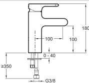
Product Specification: Single-lever basin mixer. E10496. Collection: SINGULIER. WEIGHT: 2.5 kg. MATERIAL: Metal. INSTALLATION TYPE: 1 hole. NORMS AND REGULATION: NF: I - ECAU: E1 C2 A2 U3. TYPE: Single-lever. FLOW RATE: 12 I/min. CONNECTION: With supply hoses. MECHANISM: Ceramic disc cartridge. HOLE CONFIGURATION: 180. WASTE: Without waste. MECHANISM GUARANTEE: 5 years.
