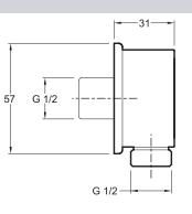
Product Specification: Shower elbow. E75142. Collection: NO COLLECTION. DIMENSIONS: 9 x 7 x 7 cm. WEIGHT: 0.3 kg. MATERIAL: Metal. INSTALLATION TYPE: 36. For directing shower hose on tap outlet, with non-return valve.
