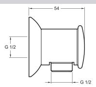
Product Specification: Elbow. E11627. Collection: NO COLLECTION. WEIGHT: 0.8 kg. MATERIAL: Metal. INSTALLATION TYPE: Wall-mount. WITH OR WITHOUT BRASSWARE: WITHOUT TAPS AND FITTINGS. Brass construction.
