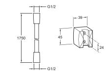
Product Specification: Shower set. E14321. Collection: ECO. WEIGHT: 1 kg. MATERIAL: Metal. INSTALLATION TYPE: Wall-mount. Shower set with fixed ABS wall support, double-interlock metallic hose 1.75 m and single-spray anti-scale handshower.
