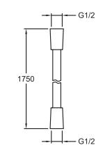
Product Specification: Shower set. E14322. Collection: ECO. WEIGHT: 1 kg. MATERIAL: Metal. Shower set double-interlock metallic hose 1.75 m and single-spray anti-scale handshower.
