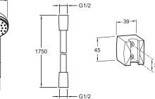
Product Specification: Shower set. E14326. Collection: BASIC 1. WEIGHT: 1 kg. MATERIAL: Metal. INSTALLATION TYPE: Wall-mount. Shower set with fixed ABS wall support, double-interlock, anti-twist hose 1.75 m and 2-spray anti-scale handshower.
