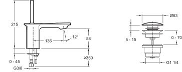
Product Specification: Single-lever washbasin mixer - "Joystick" lever. E14760. Collection: STANCE. WEIGHT: 2.8 kg. MATERIAL: Metal. INSTALLATION TYPE: 1 hole. TYPE: Single-lever. FLOW RATE: 5 l/min. HEIGHT UNDER SPOUT: 215. SPOUT PROJECTION: 136. CONNECTION: With supply hoses. MECHANISM GUARANTEE: 5 years. For water savings and comfort of use - reduced spray. Integral anti-scale aerator.
