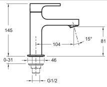
Product Specification: Pillar tap for handwash basin (cold water). E37333. Collection: STRAYT. WEIGHT: 1 kg. MATERIAL: Metal. INSTALLATION TYPE: 1 hole. NORMS AND REGULATION: ACS: 15 ACC LY 081. FLOW RATE: 5 I/min. MECHANISM: Ceramic disc valve. WASTE: Without waste. No drain. Cold water only. Anti-scale aerator.
