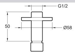
Product Specification: Arm for showerhead, overhead installation. E889. Collection: NO COLLECTION. DIMENSIONS: 2.10 x 2.10 cm. WEIGHT: 1 kg. MATERIAL: Metal. INSTALLATION TYPE: Wall-mount.
