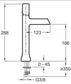
Product Specification: Tall single-lever washbasin mixer, smooth body. E8960. Collection: TOOBI. WEIGHT: 1.7 kg. MATERIAL: 54. INSTALLATION TYPE: 1 hole. TYPE: Single-lever. CONNECTION: With supply hoses. MECHANISM: Ceramic disc cartridge. WASTE : Without waste. INSTALLATION TYPE: 1 hole. MECHANISM GUARANTEE: 5 years. Flow limit 8 l/min. No waste.
