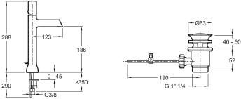
Product Specification: Tall single-lever washbasin mixer with supply hoses. E8990. Collection: TOOBI. WEIGHT: 1.9 kg. MATERIAL: 54. INSTALLATION TYPE: 1 hole. TYPE: Single-lever. FLOW RATE: 8 l/min under 3 bar. CONNECTION: With supply hoses. MECHANISM: Ceramic disc cartridge. INSTALLATION TYPE: 1 hole. MECHANISM GUARANTEE: 5 years. Flow limit 8 l/min. No waste.
