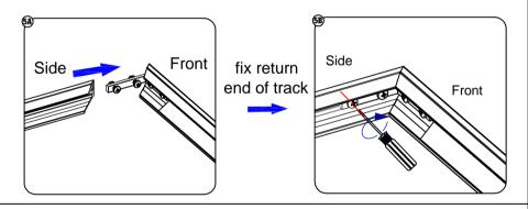
$\begin{tabular}{ll} \textbf{Step 6} & \textbf{Insert the glass fixing profile into the side section of the bottom track} \\ \end{tabular} .$
