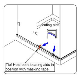
Step 23 Lift door onto locating aids and retain door into position using top holding strip
