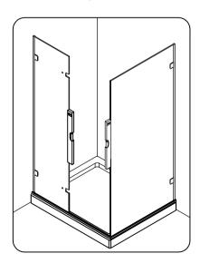
Using 4mm hex key fully tighten bracket to glass.
