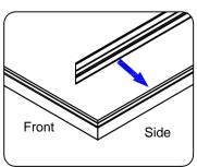
Position brackets 8mm inwards from edge of tray Mark wall through slot. Drill 6mm diameter hole centre of slot and fix bracket both sides.
