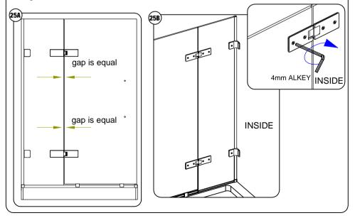
Remove top holding strip. To remove door positioning aids open door outwards. When positioning aids have been removed check gap beneath door is even.
