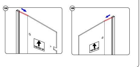
Fix wall brackets loosely ensuring fixing holes are to the inside of glass panel.
