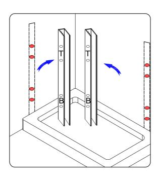
Remove profile and drill holes for wall brackets with diameter 8mm masonery bit and insert wall plugs. Ensure wall plugs are flush with tile. Repeat for each wall side panel.
