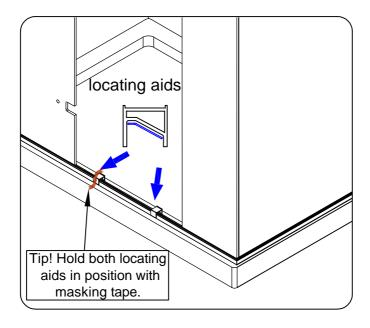
Step 30 Lift door onto positioning aids, and retain door into position using top holding strip
