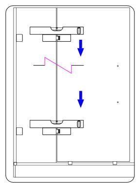
Ensure gap between both glass panels is equal top and bottom, then fully tighten hinge bolts.
