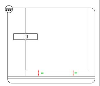
Left and right hand seal kits are provided, determine handing and use appropriate seal kit. Left hand model shown below. Push on longest seal between hinges onto back edge of moving panel. Take shortest seal and fit to top keeping notch to hinge. Repeat with longer bottom seal. Fit closing seal to edge of side panel.
