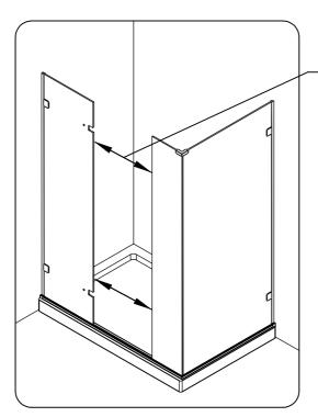
Gap top and bottom should be width of moving panel +12mm
