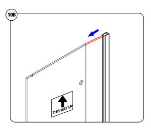
Fix wall brackets loosely ensuring fixing holes are to the inside of glass panel.
