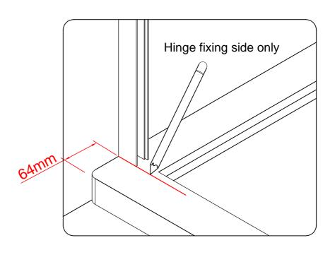
Note the position of the labels on the wall profile. Make sure Label 'T' is to the top and 'B' is to the bottom. Line up the outside edge of the profile with the mark and plumb vertical. Mark the wall through the pre-drilled holes.
