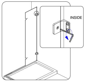
15A) Insert guide spacer to front corner of track.
