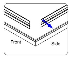
Add a dab of silicone to the back of the wall bracket and fix with 4x30 screws.
