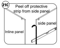
**Step 21**Firmly press along joint to ensure a watertight seal working from top to bottom.
