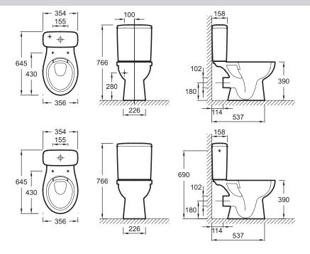
Product Specification: Rimless WC pan, P-trap. UJV101. Collection: PATIO. DIMENSIONS: 64.40 x 35.60 cm. WEIGHT: 22.1 kg. MATERIAL: Ceramic. INSTALLATION TYPE: Floor-standing. NORMS AND REGULATION: NF. VOLUME OF WATER: 2.6/4 L and 3/6 L. HEIGHT: Standard. RIM TYPE: Rimless.
