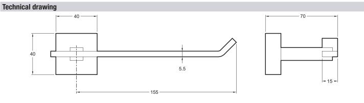
Product Specification: Toilet roll holder. E77870. Collection: E0. DIMENSIONS: 15.50 x 7 x 4 cm. WEIGHT: 0.3 kg. MATERIAL: 54. INSTALLATION TYPE: Wall-mount.
