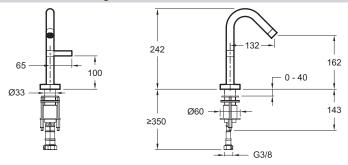
Product Specification: Single-lever basin mixer. E78130. Collection: LÉONIE. WEIGHT: 1.4 kg. MATERIAL: 54. INSTALLATION TYPE: 1 hole. TYPE: Single-lever. FLOW RATE: 6 I/mn. CONNECTION: With supply hoses. INSTALLATION TYPE: 1 hole. MECHANISM GUARANTEE: 5 years.
