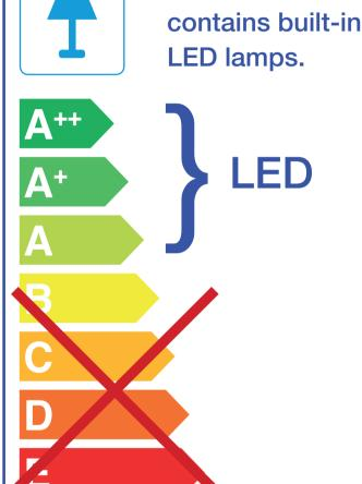
The lamps cannot be changed in the luminaire.
