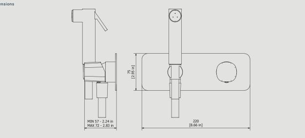
Cartridge Threaded fitting G1/2" female Ø35 ceramic cartridge Aerator Flow Rate (+/-10%) 1 BAR 2 BAR 3 BAR 2.3 I\min 3.2 I\min 4 I\min
