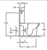
Product Specification: Rimless WC pan, vario outlet. UJN102. Collection: VOX. DIMENSIONS: 66.50 x 36 cm. WEIGHT: 30.7 kg. MATERIAL: Ceramic. INSTALLATION TYPE: Floor-standing. VOLUME OF WATER: Standard 3/6 L. HEIGHT: Comfort. RIM TYPE: Rimless. SEAT : Not included. TOILET BOWL FIXINGS: Concealed.
