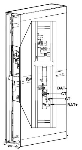
**Connect Communication Cables between the I/O Cabinet and Battery Cabinet**
