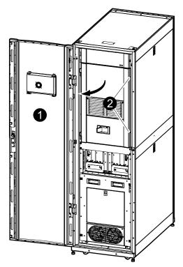
3. Remove the four screws from the air guide as shown.
