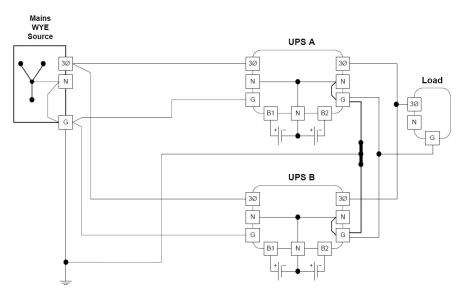
Connect an N-G bond in each UPS, and connect the UPS output neutral via tap conductors to a common grounded electrode bus and a single grounding electrode conductor. See NEC 250.30 (A)(4), including Exception #1.
