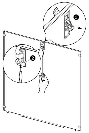
4. Take the two seismic lock parts and put them together.
