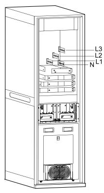
2. Install plastic covers over the output terminals L1, L2, L3.
