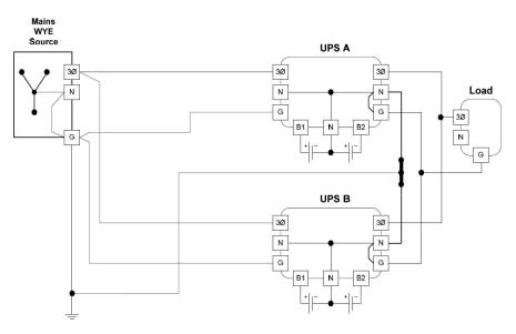
• Connect an output neutral from each UPS to a neutral/bonding bus in the maintenance bypass panel, and bond the maintenance bypass panel neutral bus to the ground with a single N-G bonding jumper and a grounding electrode conductor. See NEC 250.30 (A) Exception #1.
