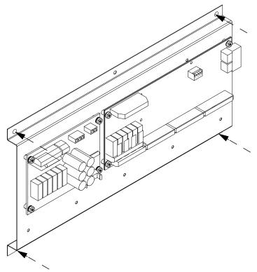
2. Attach the assembly with the four supplied M5 screws and nuts.
