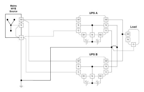
**NOTE:** Schneider Electric recommends that each UPS in the parallel system has a neutral connection installed. Contact Schneider Electric for information on other configurations.
