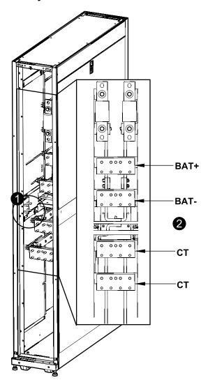
2. Connect one end of the battery cables to the BAT+, BAT-, and CT (Midpoint) cable landings in the battery side car.
