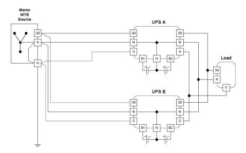
However if the load is a 3–phase load, the three alternatives below for 3–wire installations are allowed:
