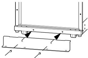
2. Bolt the front anchoring bracket to the floor using floor anchoring bolts (not supplied). Use M12 strength class 8.8 or 1/2 in grade 5 steel bolts.
