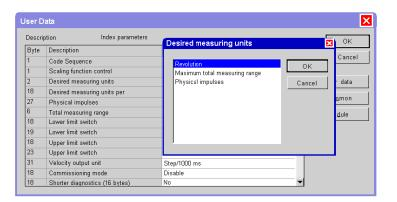
**Desired measuring units per revolution:** The position value is incremented by the number of programmed steps (desired measuring units) during a revolution. The "Total resolution" parameter is used to adapt the measuring range (see *Total measuring range*, page 41).
