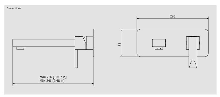
Cartridge Threaded fitting IB 35 mms Ceramics Discs Cartridge Treaded fitting G1/2" female Aerator Flow Rate (+/-10%) 1 BAR 2 BAR 3 BAR M24x1 12.3 l\m 8.8 l\m 15.2 l\m
