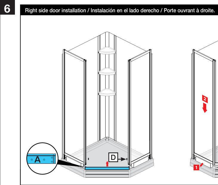
If the door will open to the left, use the support bar with label [A]. Slide it into the panels, and install and tighten the (4) M5 screws [D]. Remove the wood blocks and carefully slide the panels down.
