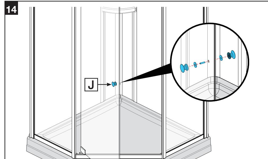
**CAUTION:** Risk of injury or product damage. During installation tempered glass should not come in direct contact with metal parts or it may shatter. Gaskets must always be used in between glass and metal. Install the handle assembly [J]. Make sure the gaskets are in place between the glass and handle knobs.
