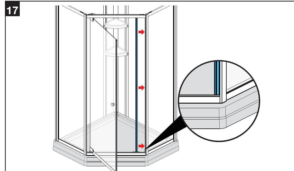
Attach strike side magnetic gasket to the stationary panel. Make sure that the bottom of the magnetic gasket touches the bottom support bar.
