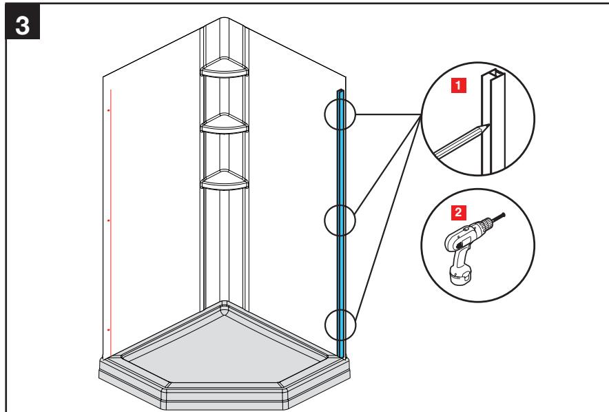
Position the wall jamb so that it is lined up with the marked line. Mark (3) holes locations for each wall jamb and remove the wall jamb. Drill holes through wall material using a 3/16" drill bit (for tile walls, use a glass and tile bit). Then use a 7/64" drill bit to drill holes into studs, or insert (6) anchors [K] into holes and tap into place with a hammer.
