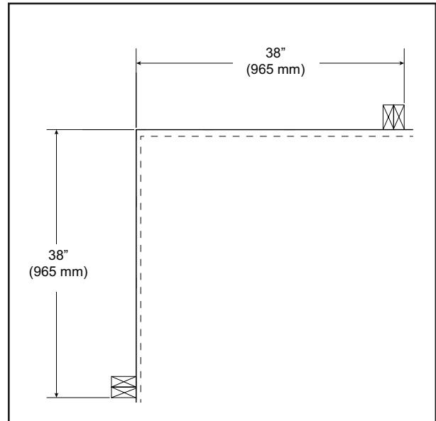
Studs must be in this location on each side for enclosure installation. Other stud locations are not critical.
