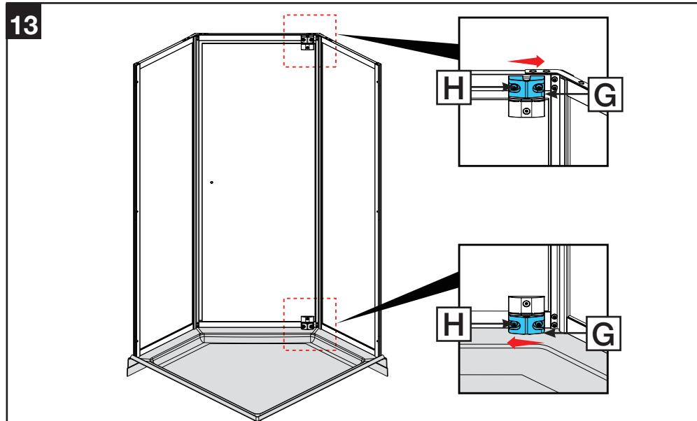
Move the top and bottom hinge bushings [G] from left to right to level the door. After adjustments have been made, tighten all (4) M6 screws [H].
