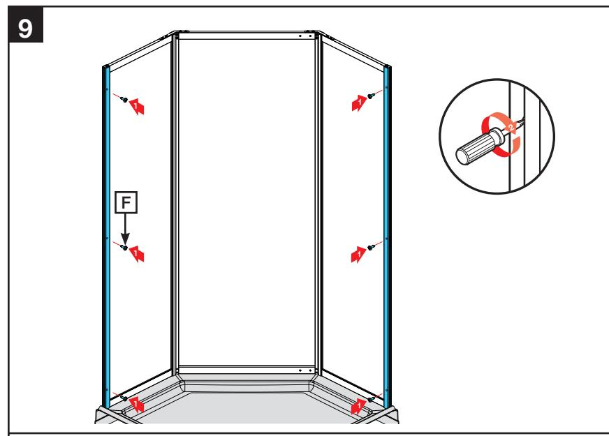
Secure the panels to the wall jambs using (6) M4 screws [F].
