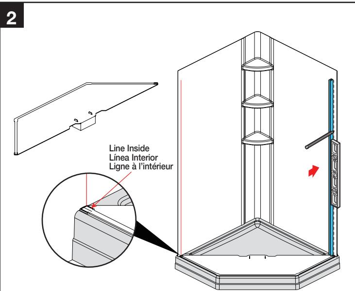
Fold the install template as shown. Place the template on the base and adjust it so that the edges are even with the base, and the template is touching both finished walls. Transfer the wall jamb inside edgeline from the template to each wall. Using a long level, extend plumb lines up the wall.
