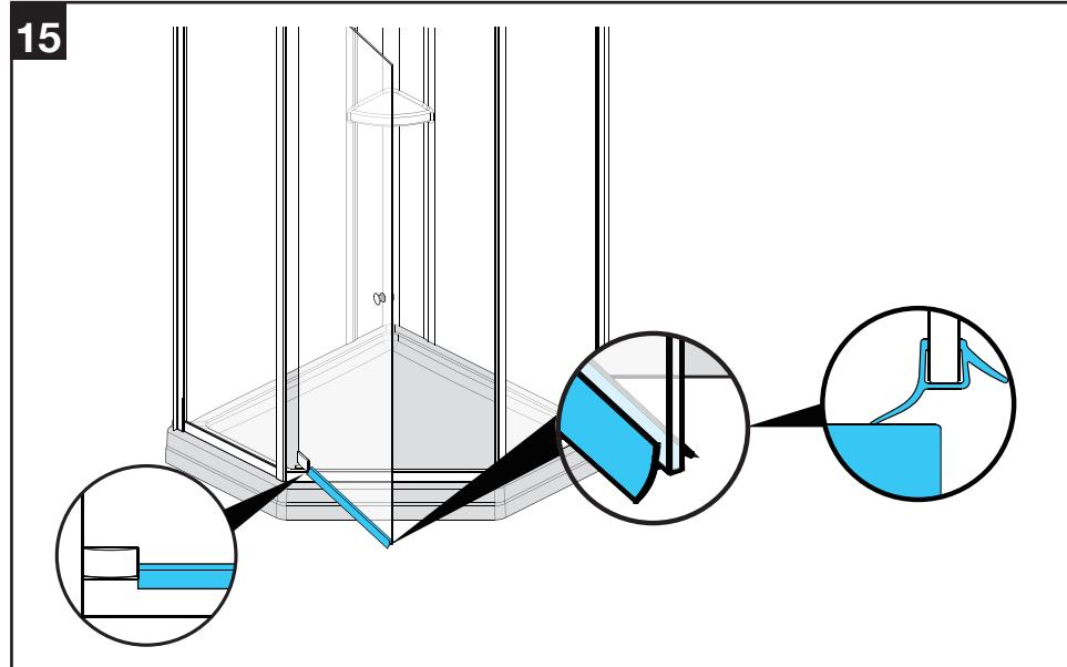
Attach door sweep gasket to the bottom of door. Make sure that the end of the gasket touches the hinge plate. The long fin is on the outside.
