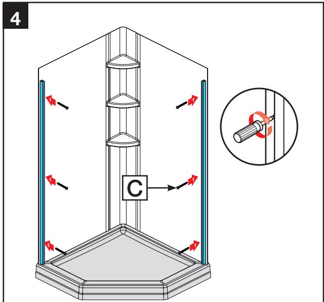
**CAUTION:** Screws must go into studs, if not using anchors. Install wall jamb using (6) M4 x 50mm screws [C].
