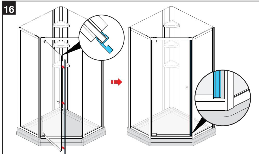
Attach magnetic door gasket to door. Make sure that the bottom of the magnetic gasket overlaps the sweep gasket. NOTE: The bottom of the magnetic gasket should leave a small gap at the bottom support bar when the door is closed.
