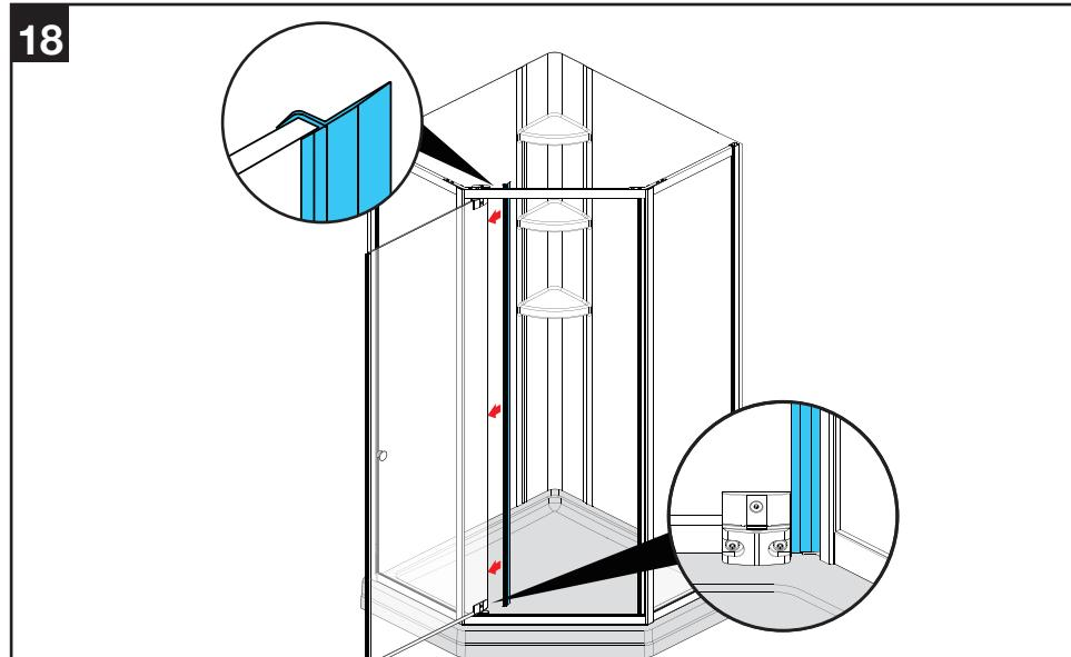
Attach hinge side gasket to door. Make sure that the bottom end of the gasket is lower than the top surface of bottom support bar.
