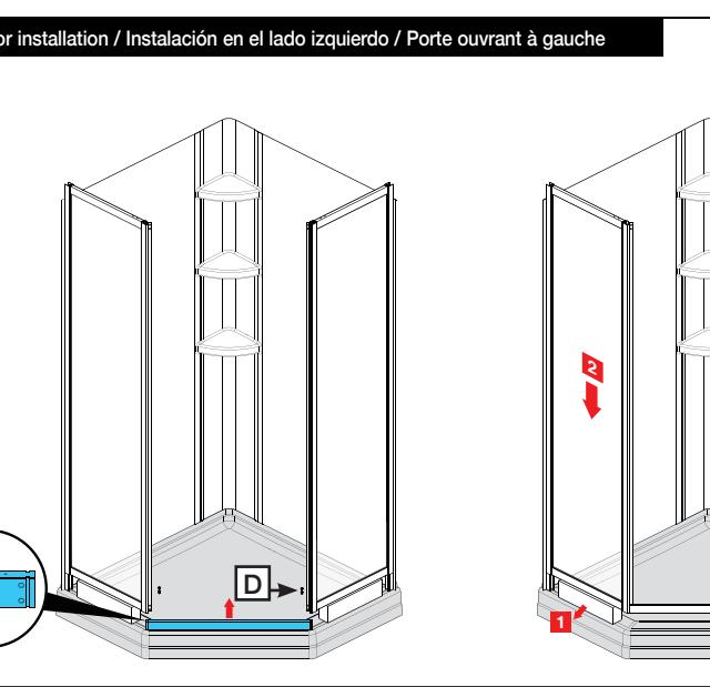
If the door will open to the right, use the support bar with label [B]. Slide it into the panels, and install and tighten the (4) M5 screws [D]. Remove the wood blocks and carefully slide the panels down.
