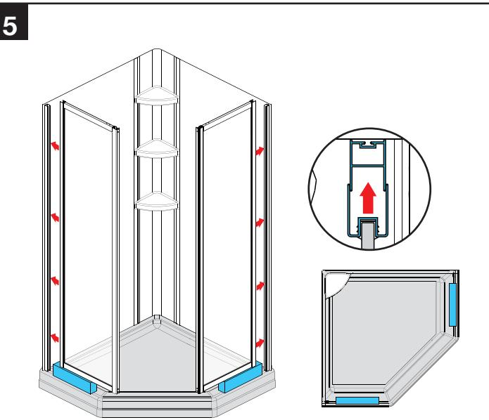
Insert the glass panels over the wall jambs and rest on wood blocks.
