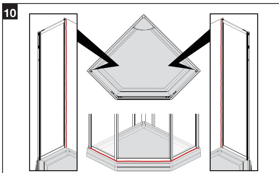
Apply sealant to the outside bottom of the support bar and panels, the inside of wall jamb.
