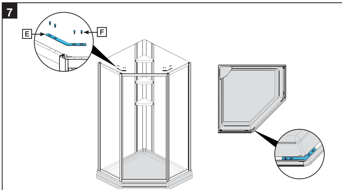
Install the angle bracket [E]. Secure the brackets to the support bar and panels using (8) M4 screws [F]. NOTE: Check that the glass panel is even with the edges of the base before tightening the M4 screws [F].
