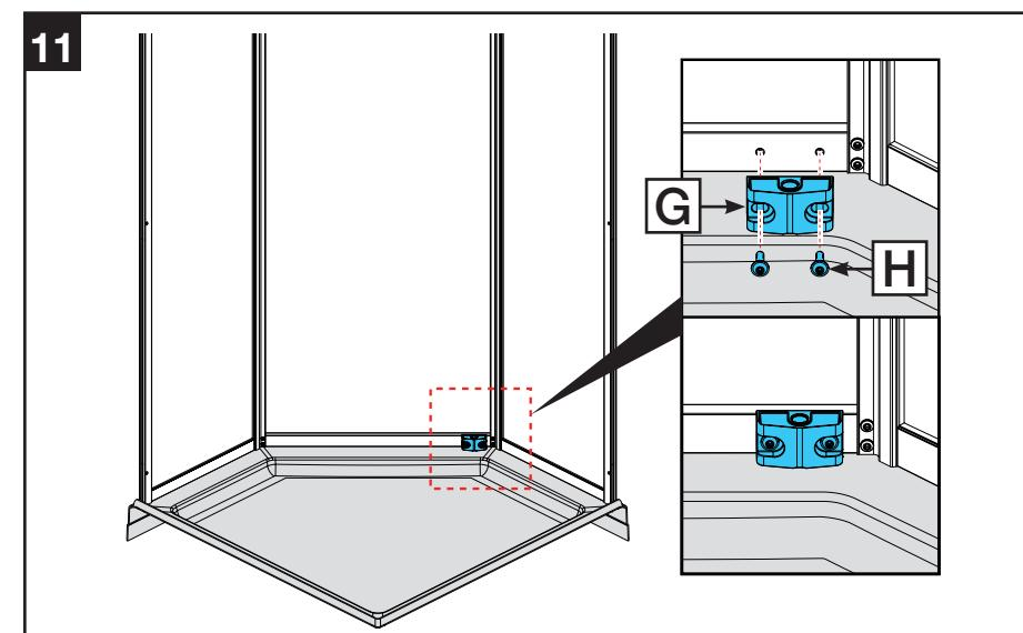
Install the hinge bushing [G] onto bottom support bar using (2) M6 screws [H].
