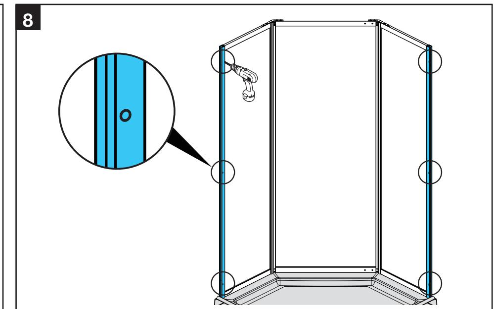
From inside the shower, drill three pilot holes through the panel into each wall jamb using 1/8" drill bit.
