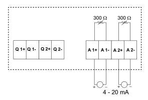
You can configure the following analog inputs on your meter through communication only:
