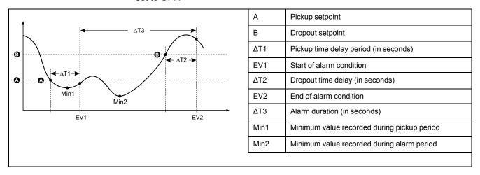
The meter records the date and time when the alarm event starts (EV1) and when it ends (EV2). The meter also performs any task assigned to the event, such as operating a digital output. The meter also records minimum values (Min1, Min2) before, during or after the alarm period.
