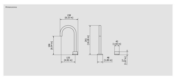
Cartridge Threaded fitting G1/2" female 400mms Ø25 progressive cartridge Aerator Flow Rate (+/-10%) 1 BAR 2 BAR 3 BAR M16.5x1 3 I\m 3.8 l\m 3.8 l\m
