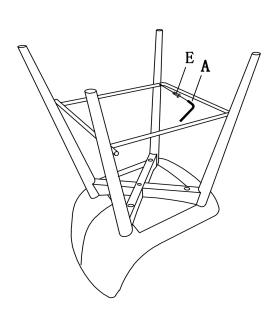
Tip: tighten all screws after the footrest is assebmled!
