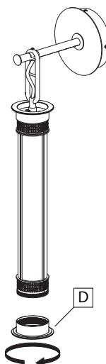
**EN** Unfasten the end cap (D) from the main body. Install the diffuser and then re-fasten the end cap (D) to secure it. Remove the locking screw and protecting piece (E).
