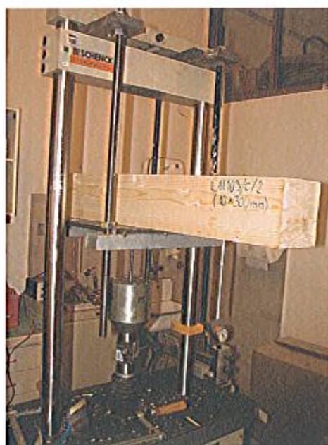
Figure 6: Withdrawal parameter test – testing equipment (1)
