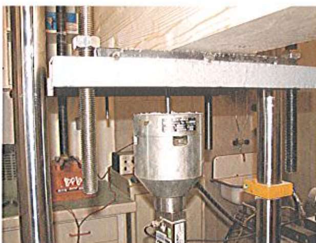
Figure 8: Withdrawal parameter test – testing equipment (3)
