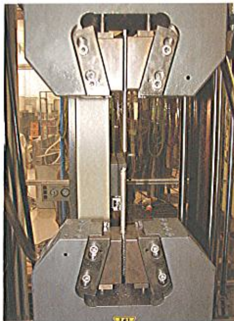
Figure 13: Tensile strength test ( d = 12 mm)
