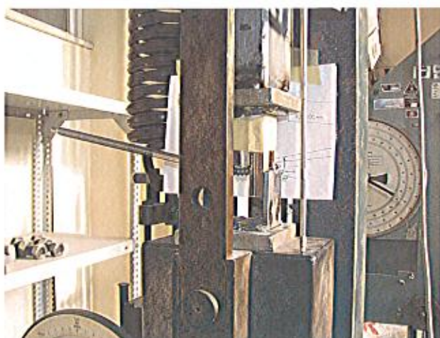
Figure 5: Yield moment test: Test on threaded part of screw
