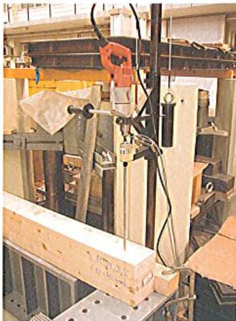
Figure 9: Torsional resistance to insertion of screws – testing equipment
