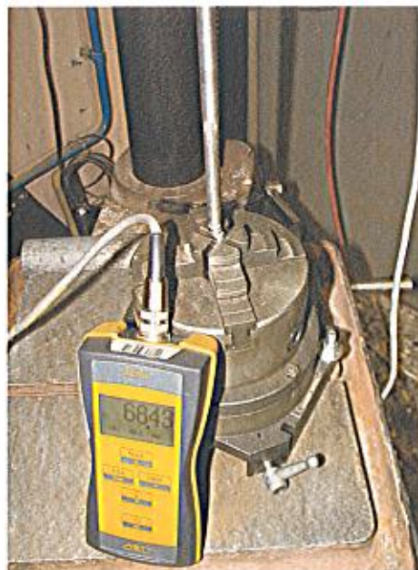
Figure 11: Torsional strength test - detail
