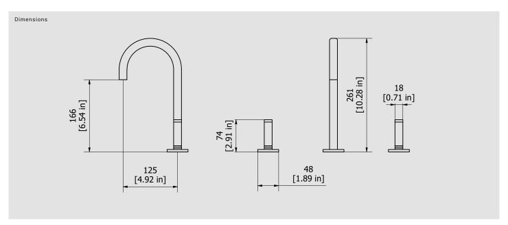
Cartridge Threaded fitting G3/8" ceramic headwork Inox hose G1/2" male Aerator Flow Rate (+/-10%) 1 BAR 2 BAR 3 BAR M16.5x1 3 I\m 3.8 I\m 3.8 l\m
