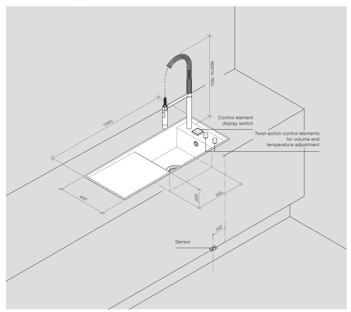
The sink-integrated eUNIT KITCHEN involves a predefined product configuration. Electronic control elements are already pre-fitted on the single sink.
