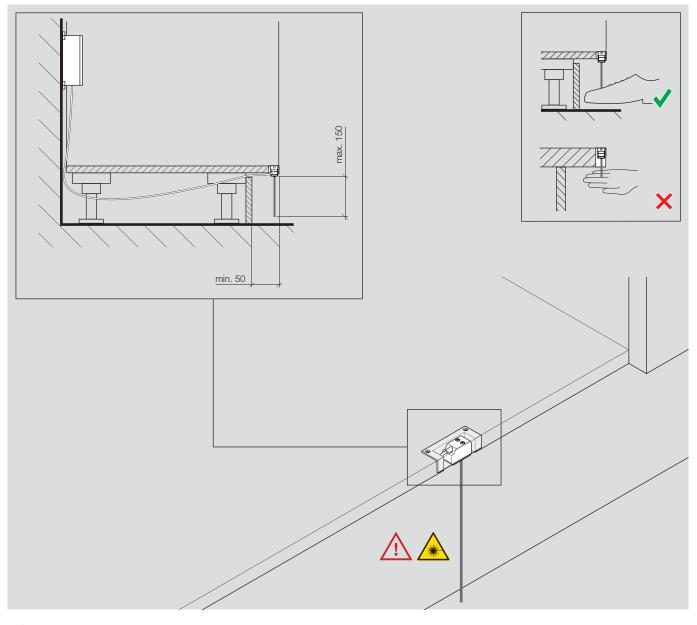
The sensor used is a Class 1 laser product, with a very low output (40 µW for blue light). This laser product meets the requirements of DIN EN 60825-1 / IEC 60825-1:2007. The accessible laser beam is not dangerous under the conditions that might reasonably be anticipated. The laser product must be installed in such a way that the only way to operate it is by using your foot.
