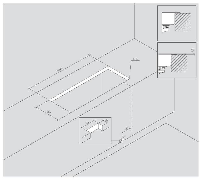
The thickness of the worktop in the sink cutout area must not exceed 50 mm. A relevant cutout template and installation instructions with details for sink mounting are included with eUNIT KITCHEN.
