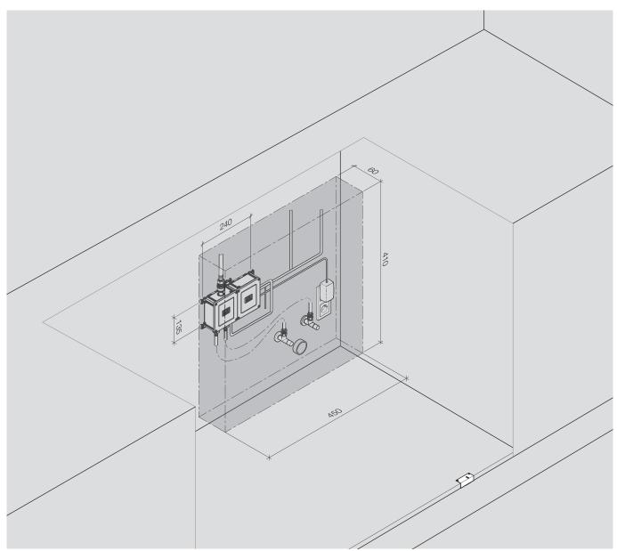
This installation example shows the minimum space requirement for the control unit and connection components.
