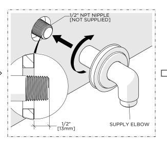
Ensure the 1/2" NPT NIPPLE (not supplied) is 1/2" [13mm] from the surface of the finished wall then thread and securely tighten the ELBOW onto the NIPPLE.
