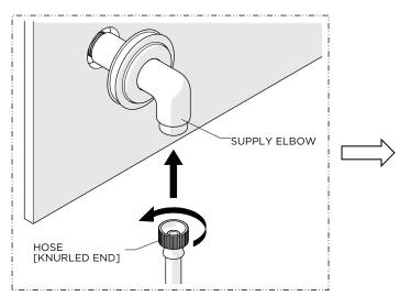
7. Thread and securely tighten the knurled end of the HOSE to the ELBOW.
