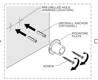
Using the previous marks as a reference, install the MOUNTING PLATE using the ANCHORS (if needed) and WOOD SCREWS provided.
