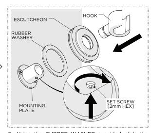
Using the RUBBER WASHER provided, slide the ESCUTCHEON back onto the MOUNTING PLATE then insert the HOOK back into the PLATE and securely tighten the SET SCREW.
