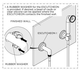
10. Slide the ESCUTCHEON down the ELBOW until it contacts the finished wall.
