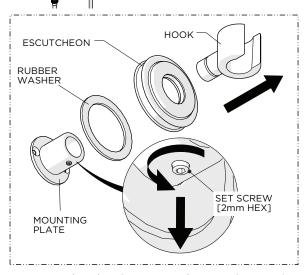
Loosen, but do NOT remove, the SET SCREW using a 2mm HEX KEY then remove the HOOK, ESUCTCHEON and RUBBER WASHER from the MOUNTING PLATE.
