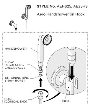
Thread and securely tighten the conical end of the HOSE to the HANDSHOWER then place it into the HOOK.
