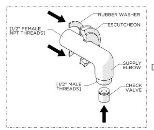
Slide the ESCUTCHEON and RUBBER WASHER onto the SUPPLY ELBOW.
