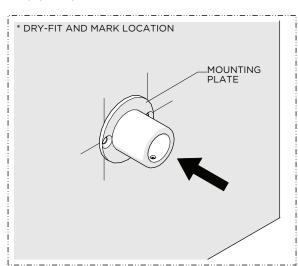
Dry-fit the MOUNTING PLATE to the finished wall and mark the ideal location for installation; preferably over adequate blocking or stud material.
