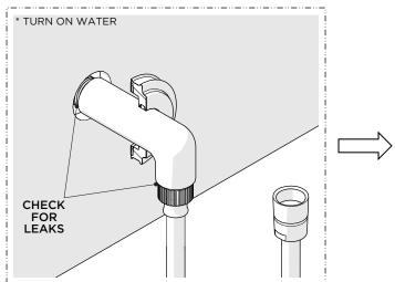
Turn on the water and a diverter/wall valve (sold separately) to flush out any debris in the supply line and inspect all connections for leaks then turn the water off.
