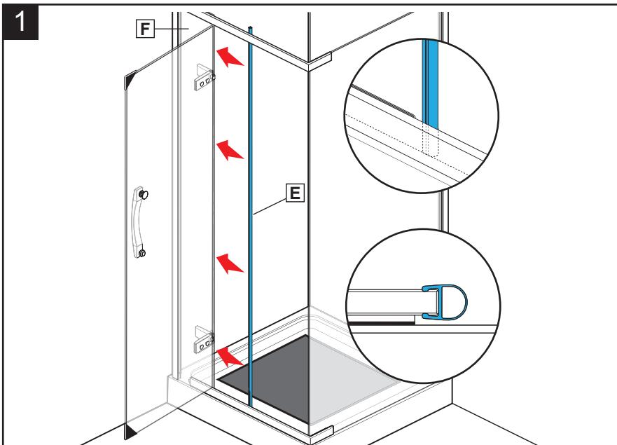
Starting at the bottom, press the bulb gasket (E) onto the edge of the small glass panel (F).
