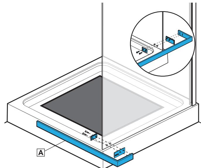
Install bottom glass support bar (A) using the plastic spacer on the outside of the glass. Use the metal bracket on the inside of the glass. Check that the support bar is parallel with the edge of the base.
