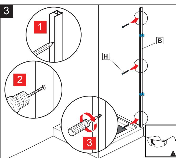
Mark (3) hole locations and remove the wall jamb (B). Drill holes through wall material using a 3/16" drill bit (for tile walls, use a glass and tile bit). Then use a 9/64" drill bit to drill holes into studs. Install wall jamb using (3) M4 x 38mm screws (H).
