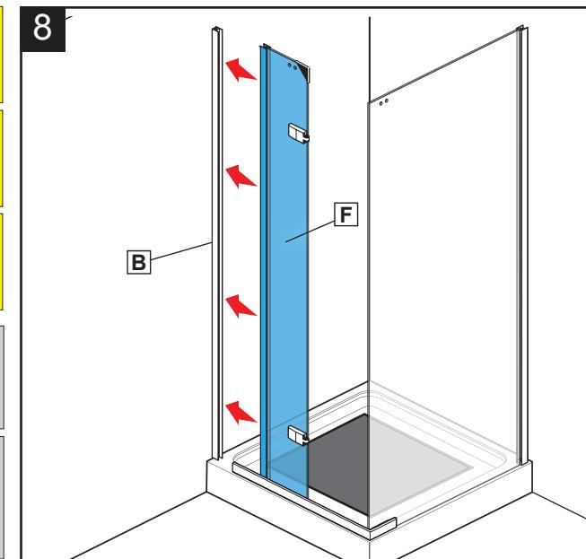
Insert the small glass panel (F) over the wall jamb (B).
