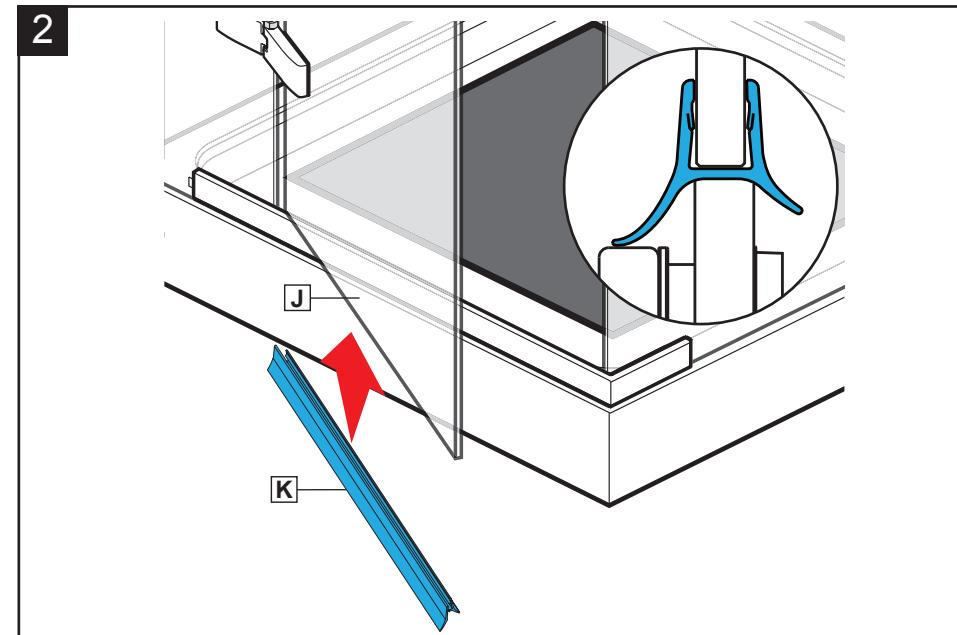
Starting on one end, press the sweep gasket (K) onto the bottom of the door (J). Make sure the ends of the gasket are flush with the glass.
