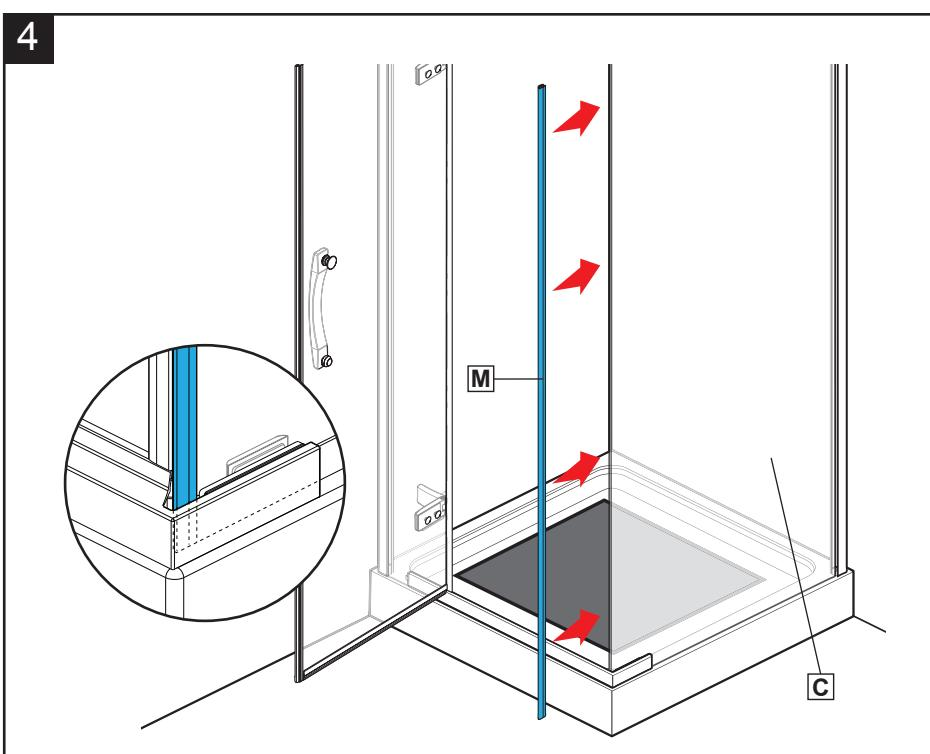
Starting at the bottom, press the magnetic gasket (M) onto the edge of the large glass panel (C).
