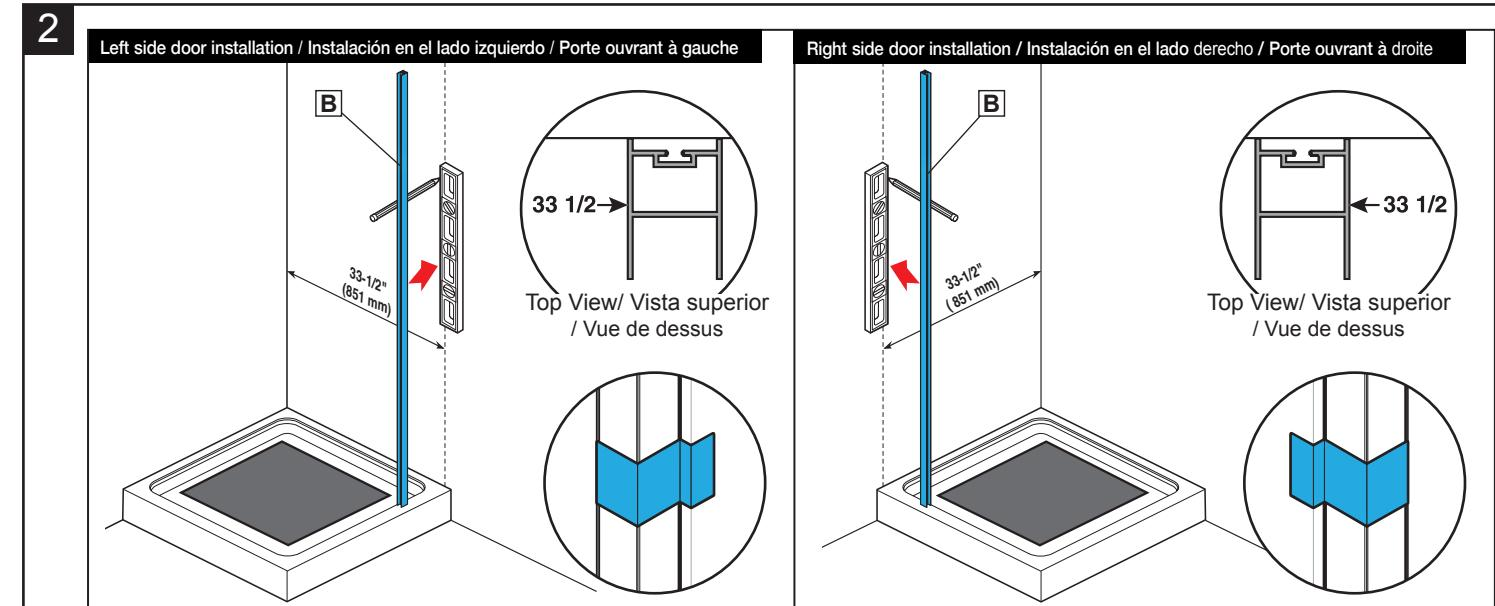
The wall jamb (B) for the large glass panel will be installed first. Measure 33 1/2" from the opposite finished wall and mark a line. Using a long level, extend a plumb line up the wall. Position the wall jamb so that the inside edge is even with the marked line. Hold it in place with tape. Check that the wall jamb is plumb.
