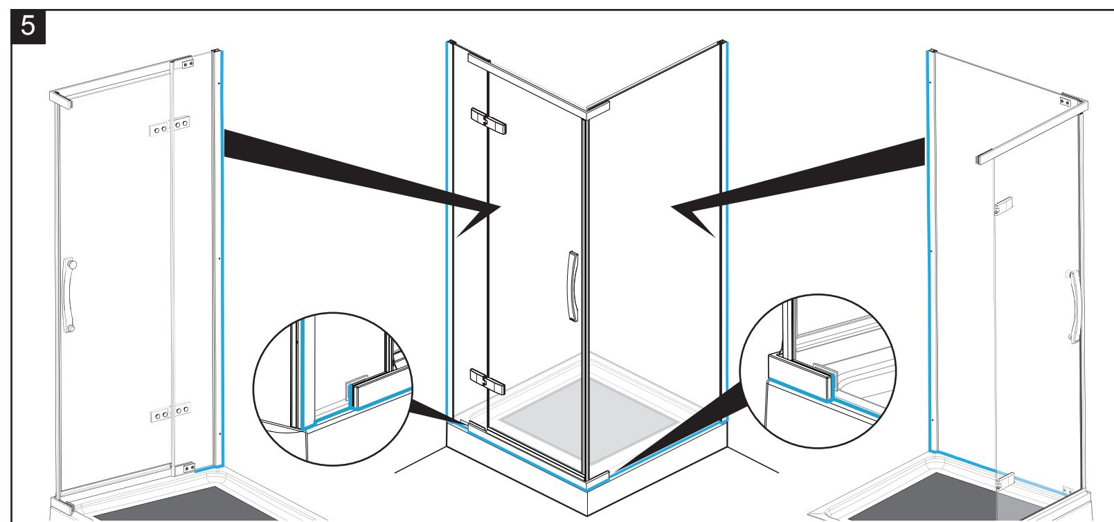
Apply sealant to both inside and outside of glass panels and support bar as shown.
