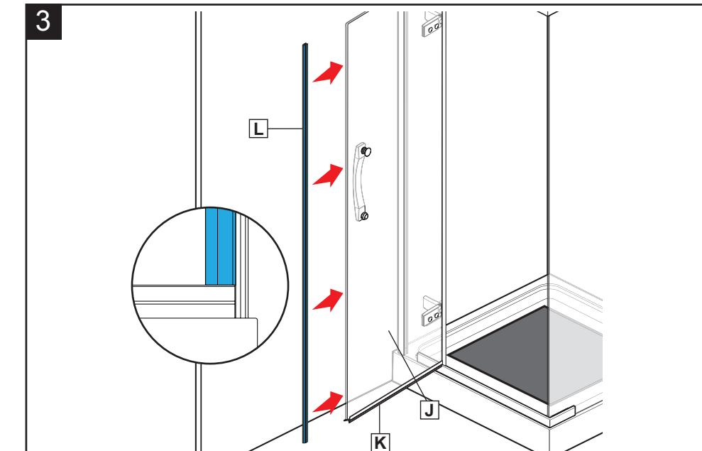
Starting at the bottom, press the magnetic gasket (L) onto the edge of the door (J). Make sure there is no gap between the bottom of gasket (L) and gasket (K).
