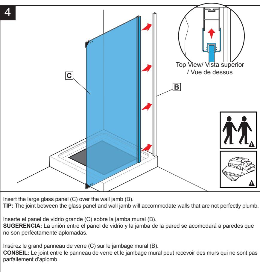
Insert the large glass panel (C) over the wall jamb (B).
