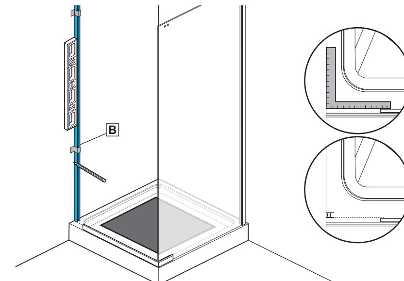
Place a framing square on the base, lined up with the support bar and opposite wall. Make sure that the support bar is even with the front edge of the base, and mark a line on the wall.
