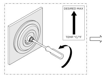
10. With water running, rotate the SQUARE TUBE to adjust the temperature to the maximum desired bathing temperature, verified with a thermometer. Turn the water off and make sure not to change this setting.
