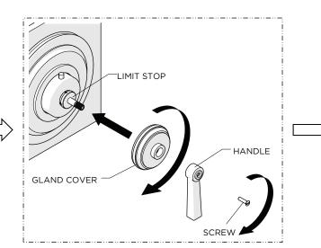
14. Thread the BUSHING back onto the LIMIT STOP, place the GLAND COVER onto the LIMIT STOP, place the HANDLE onto the STEM in the desired orientation, then thread and securely tighten the SCREW.
