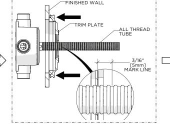
2. Firmly holding the PLATE against the finished wall, mark the TUBE 3/16" [5mm] beyond where it protrude from the PLATE.
