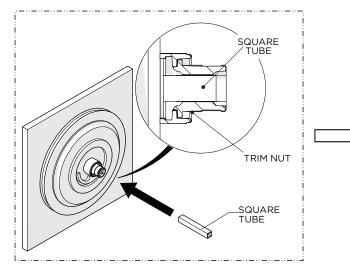
7. Re-insert the SQUARE TUBE back into the TRIM NUT making sure it is slight recessed.
