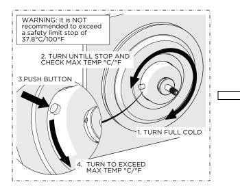
13. Turn the LIMIT STOP to cold then hot and confirm it is functioning properly. Verify the maximum desired bathing temperature. To get a hotter temperature, press and hold the LIMIT STOP BUTTON and turn the LIMIT STOP further.
