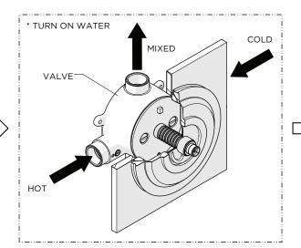
8. Turn on the water supply and open a diverter or wall valve (sold separately) to run water through the thermostatic valve.
