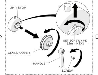
11. Unthread the SCREW, remove the HANDLE, remove the GLAND COVER then loosen the SET SCREWS (x4) using a 2mm HEX KEY.
