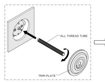
1. Thread the ALL THREAD TUBE onto the CARTRIDGE then slide the TRIM PLATE over the TUBE.
