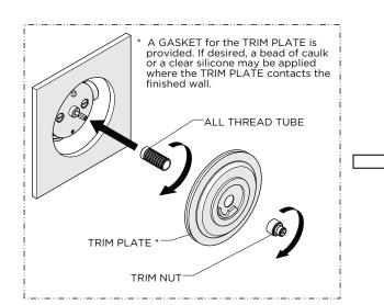
4. Thread the TUBE back onto the CARTRIDGE, slide the PLATE over the TUBE, and thread the TRIM NUT onto the TUBE. Securely tighten to hold the PLATE against the finished wall. [SHOULD FEEL RESISTANCE]
