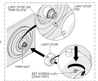
12. Place the LIMIT STOP over the TRIM NUT making sure the LIMIT STOP PIN makes contact with the LIMIT STOP on the TRIM PLATE then tighten the SET SCREWS.
