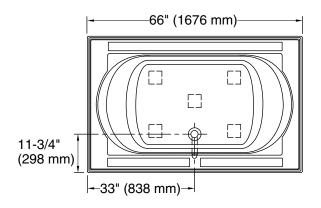
No change in measurements if connected with drain illustrated. (K-7161-AF)
