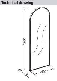
Product Specification: Vertical mirror MDF. EB1434. Collection: NO COLLECTION. DIMENSIONS: 40 x 2 x 120 cm. WEIGHT: 6.3 kg. MATERIAL: Lacquer. INSTALLATION TYPE: Wall-mount.
