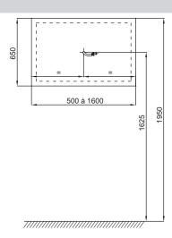
Product Specification: Mirror 60 cm - LED lighting and anti-steam. EB1470. Collection: NO COLLECTION. DIMENSIONS: 60 x 3.40 x 65 cm. WEIGHT: 6.6 kg. MATERIAL: Glass. INSTALLATION TYPE: Wall-mount.
