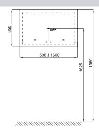
Product Specification: Mirror with LED lighting and anti-steam 140 cm. EB1476. Collection: NO COLLECTION. DIMENSIONS: 140 x 3.40 x 65 cm. WEIGHT: 12 kg. MATERIAL: Glass. INSTALLATION TYPE: Wall-mount.
