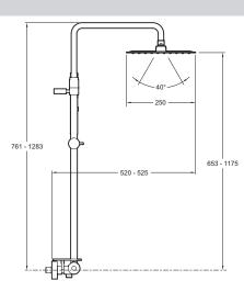
Product Specification: Thermostatic shower column. E26595. Collection: MÉTRO. DIMENSIONS: 33.40 x 33.40 x 131.50 cm. WEIGHT: 5.6 kg. MATERIAL: Metal. INSTALLATION TYPE: Wall-mount.
