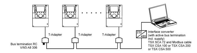
2. Using the optional Modbus splitter or an external junction box
