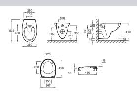
Product Specification: Suspended WC pack. EDV114. Collection: PATIO. DIMENSIONS: 53.50 x 36 cm. WEIGHT: 15 kg. MATERIAL: Ceramic. INSTALLATION TYPE: Wall-hung. VOLUME OF WATER: Standard 3/6 L. HEIGHT: Standard. RIM TYPE: Rimless. SUPPLIED WITH: Thermoset seat, metal hinges E4303-00.
