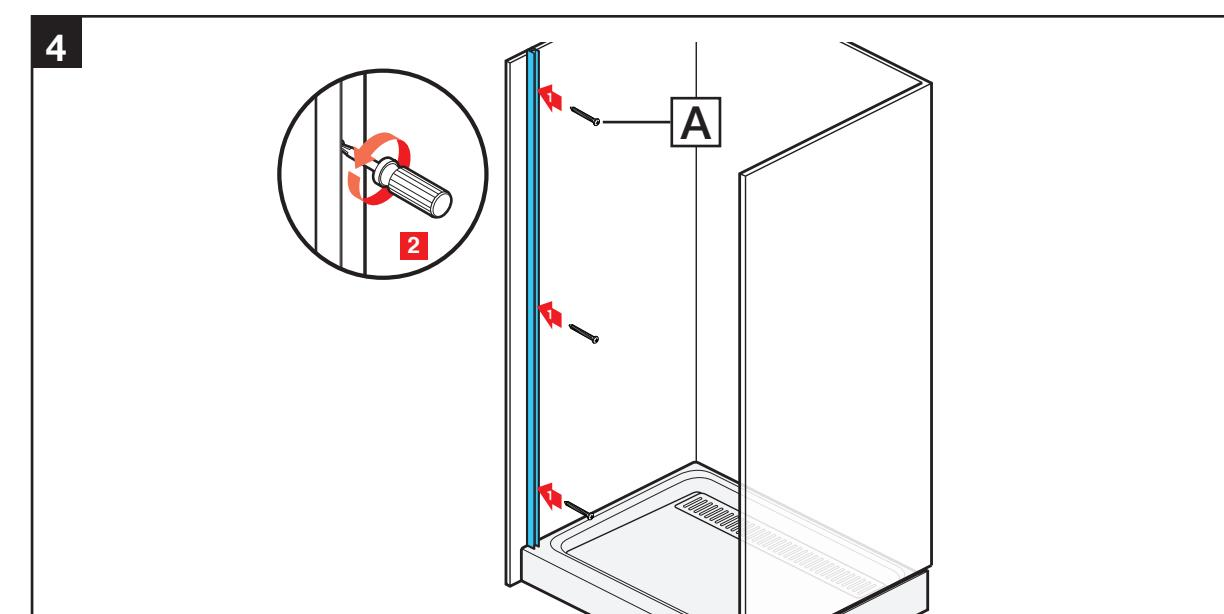
**NOTICE: Screws must go into studs.**
