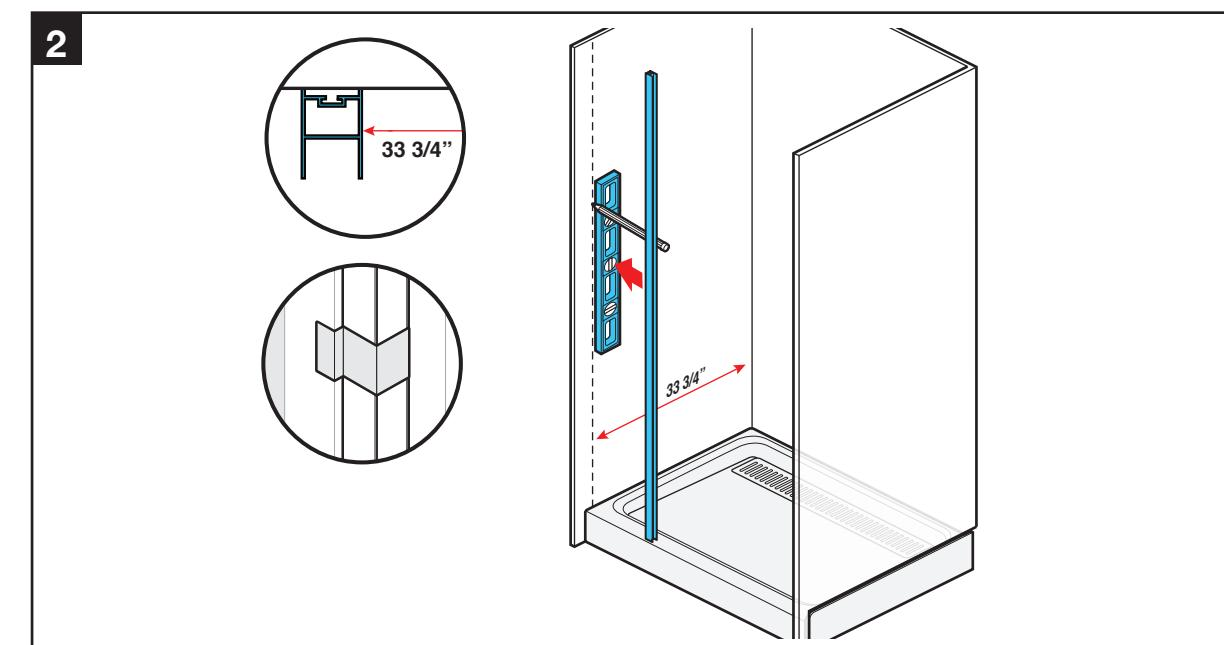
**Measure 33-3/4" from the finished back wall and mark a line.** Using a level and wall jamb, extend a plumb line up the wall.
