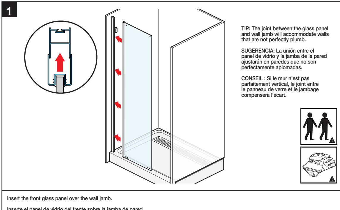
**TIP:** The joint between the glass panel and wall jamb will accommodate walls that are not perfectly plumb.
