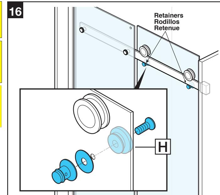
Install door retainers [H]. Do not tighten completely until after any height adjustments have been made.
