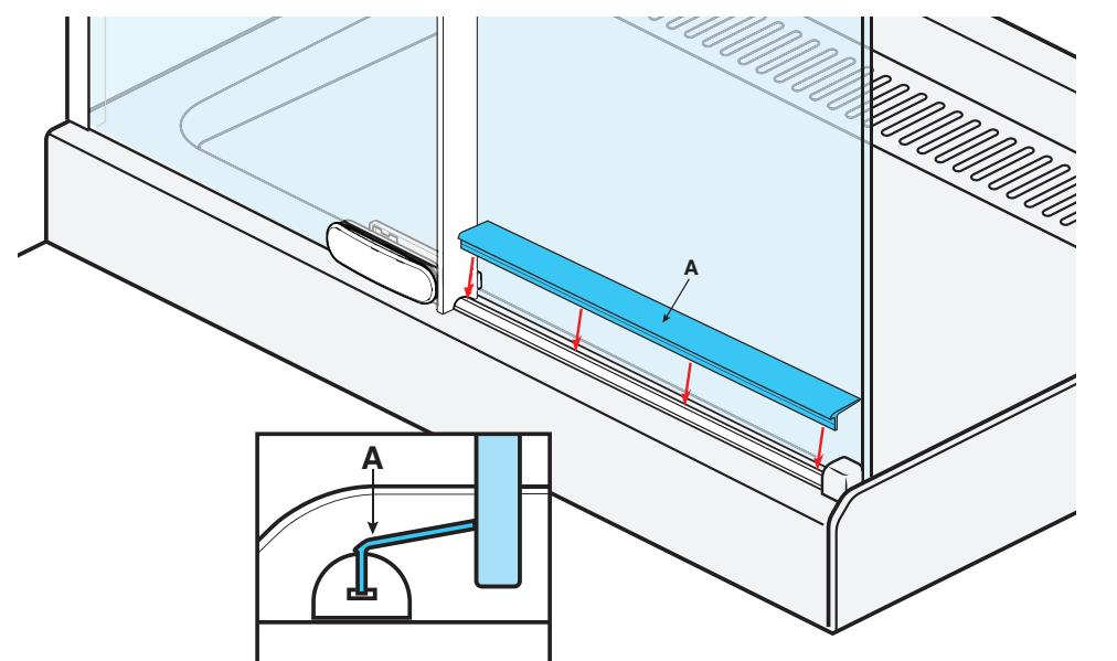
Slide the gasket A into the threshold bar against the panel gasket.
