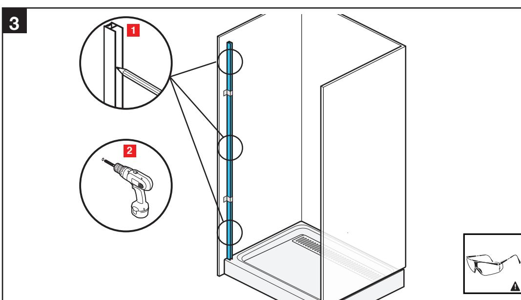
**Drill all 3 holes through wall material using a 3/16" drill bit (for tile walls, use a glass and tile bit).**
