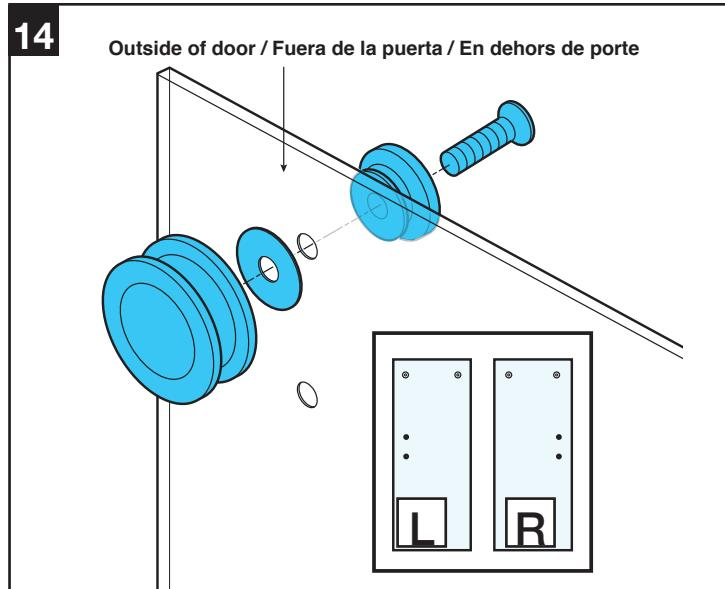
Install rollers. Do not tighten completely until after any height adjustments have been made.
