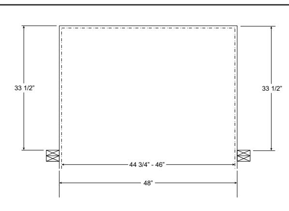
Studs must be in this location on each side for door installation. Other stud locations are not critical.
