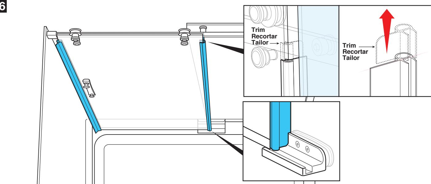
Install door gaskets. Trim inner gasket as shown.
