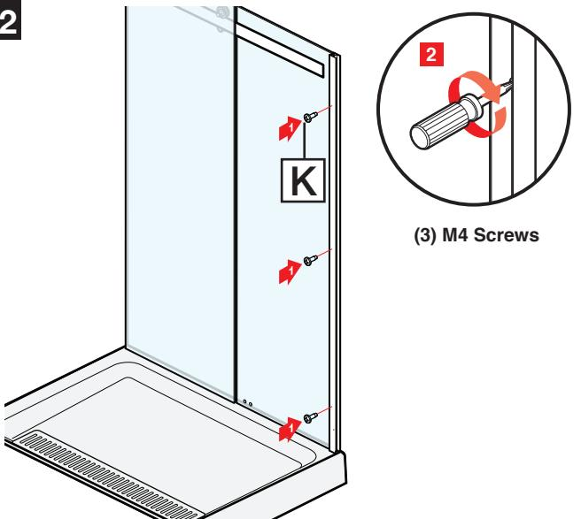
Secure the glass panel frames to the wall jambs using (3) M4 screws [K].
