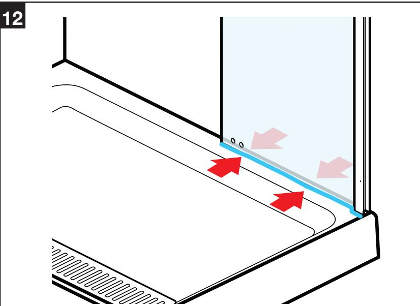
Apply sealant to the inside and outside bottom of the glass panel and wall jamb.
