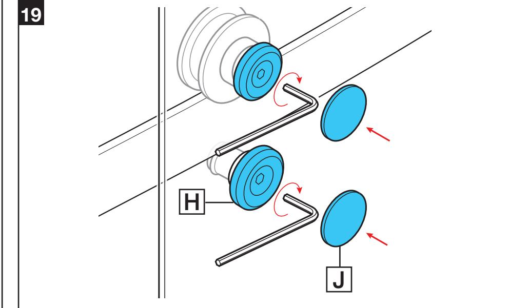
After all adjustments have been made, tighten the rollers and retainers [H]. Install caps [J].
