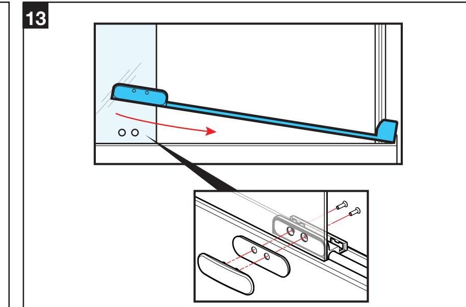
Starting with the corner side, lower the assembly into position. Tighten wall mount set screw. Then install foam gasket and door guide plate. Tighten screws.
