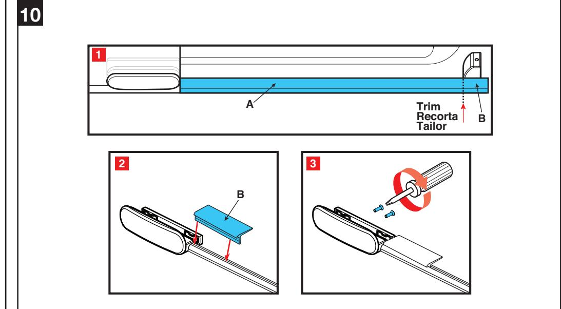
Place the threshold gasket between the door guide and lower wall mount. Trim the gasket to fit. Gasket A will be used in later step. Slide gasket B into the threshold bar against the door guide to set position. Untighten the door guide and lower wall mount.
