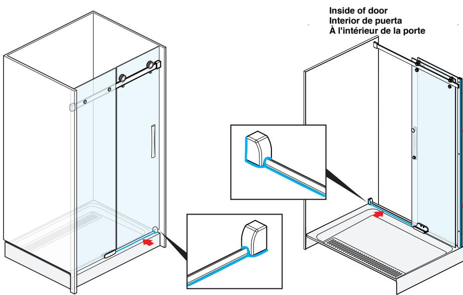
Apply sealant to threshold bar and wall mount as shown. Apply sealant where the wall jamb meets the wall inside.
