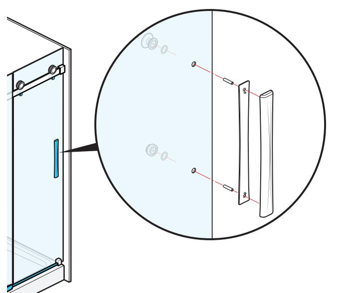
Install handle. Make sure that O-rings are in place on the inside of the door.
