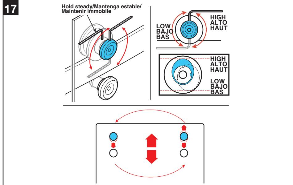
Adjust rollers up or down so door aligns with wall or glass.
