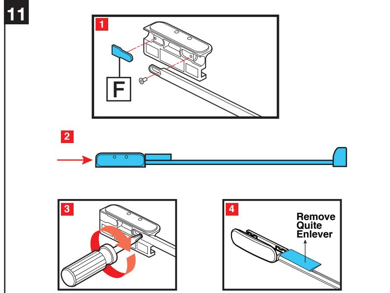
Install plug [F] and threshold bar into door guide. Slide door guide up against the gasket B and tighten the screw. Remove the gasket B. Gasket B is no longer needed and can be discarded.
