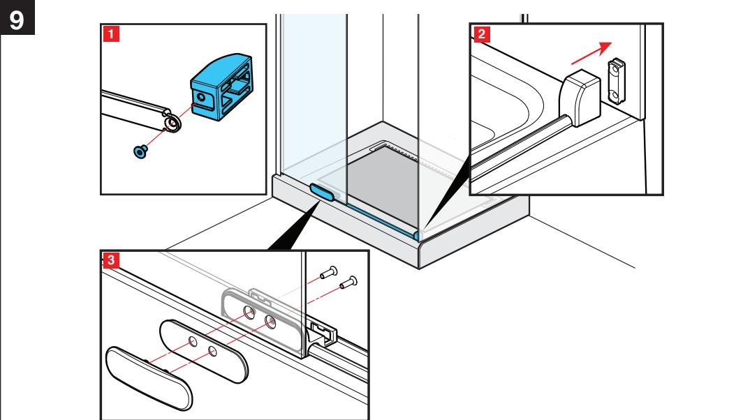
Tighten the threshold bar and the lower wall mount. Dry fit the lower wall mount and door guide. Do not completely tighten screws in step 3.
