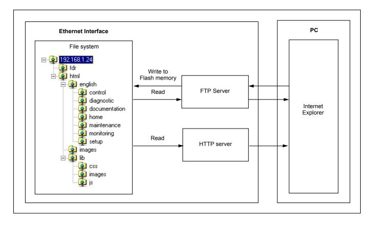
The Ethernet interface incorporates an FTP server that authorizes access to the various URLs available for the HTTP server. A browser, such as Internet Explorer, can be used to display the URLs as a disk in Windows explorer. This "disk" consists of various directories containing the URL files. It is therefore possible to use the different commands managed by the explorer such as deletion, renaming or writing (downloading) files (check that IO Scanning has been disabled on the interface).
