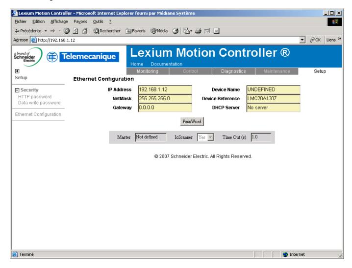
All modifications are protected by the Write password modification password. Click on the "PassWord" button to enter the Write password. After correctly entering the password, you can access "IoScanner", "Time Out (s)", "Master", "Output parameters", "Input parameters", and the "Save" and "Abort" buttons.
