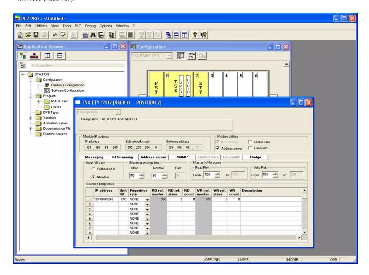
The addresses for the PLC % MW words correspond to the configuration in the previous example.
