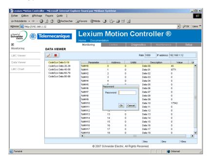
It is only possible to modify the parameter values after entering the Write password (see section entitled ""HTTP password" and "Data write password" pages", page 37). After entering the password, press the Enter key so that it is taken into account by the Web browser. When a parameter value cannot be modified, a warning message appears: "This parameter can't be written!"
