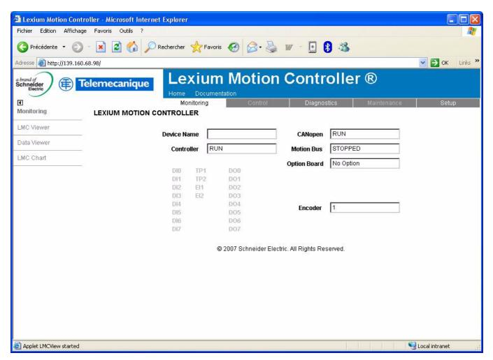
The status indicated in the "Controller" field corresponds to that of the Lexium Controller. A delay may sometimes be noticed between the displays on the Web server depending on the performance of the computer used to display the pages using a Web browser and the communication system performance.
