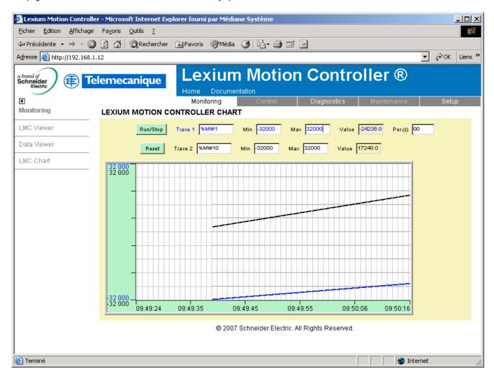
Two parameters can be selected and displayed simultaneously. To do this, select them in the Trace1 and Trace2 list.
