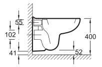
Product Specification: Wall-hung WC pan. E4345. Collection: BRIVE. DIMENSIONS: 52 x 36 cm. WEIGHT: 14.5 kg. MATERIAL: Ceramic. INSTALLATION TYPE: Wall-hung. VOLUME OF WATER: 2.6/4 L and 3/6 L. HEIGHT: Standard. RIM TYPE: Open (traditional). RIM: With rim. Semi-skirted bowl.
