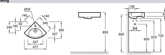
Product Specification: Corner handwash basin 34 cm. EGP112. Collection: ODÉON RIVE GAUCHE. DIMENSIONS: 34 x 34 cm. WEIGHT: 7.2 kg. MATERIAL: Ceramic. INSTALLATION TYPE: Self-supporting or can be mounted on a specific cabinet.
