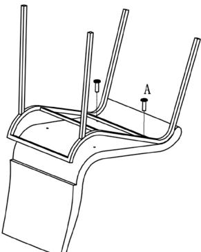
Note: For Step1, lean the chair frame a little first as the illustration, press chair frame and pre-tighten the front two screws(A). Not let the screws be tightened until Step2 finished.
