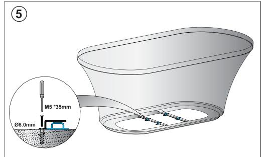
• All four floor brackets should face the same direction to allow the Surround to slide underneath during final installation.
