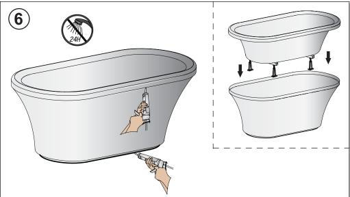
Once the overflow waste and taps have been fitted. The edge between the rim and the Surround should be sealed with a bead of clear silicon.
