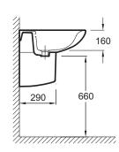
Product Specification: Washbasin. E4158. Collection: PATIO. DIMENSIONS: 55 x 45 cm. WEIGHT: 12.9 kg. MATERIAL: Ceramic. INSTALLATION TYPE: Self-supporting. FIXINGS: 2 bolts, not supplied. TAP DRILL-ING: 1 tap hole. INSTALLATION: STANDARD.
